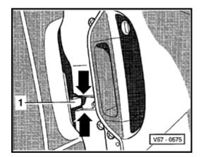
Adjust striker -1- so recess on door lock turn clip is concentric -arrows- to striker (door must not be raised or pressed down). Door must not move when closed.
