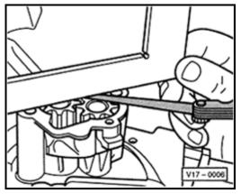
Fig. 2 Oil pump axial clearance, checking
