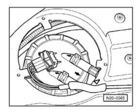
Fig. 1 Fuel delivery unit/flange, installed position
