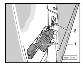
Remove remote control lock -1- by removing screws and disconnecting pull rod -2- at remote control.
