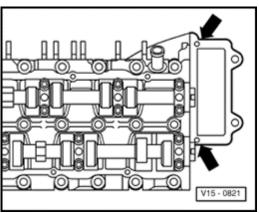
Fig. 2 Cyl. head gasket, preparing for assembly
