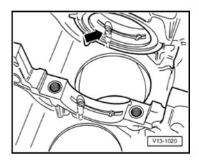
Fig. 1 Oil spray jet, removing and installing
