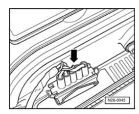
Disconnect 5-pin harness connector from ignition coil.
