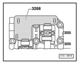
If TDC cyl. 1 setting is correct, a notch is visible on intermediate shaft sprockets -arrow-.
