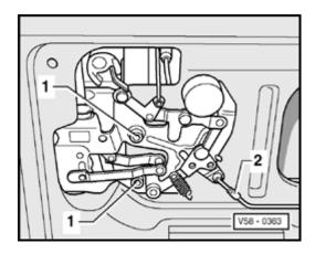
Remove Bolts and disconnect pull rod -2-. Push remote control to one side.
