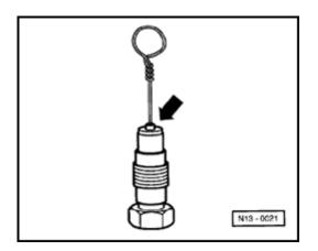
Fig. 3 Chain tensioner for double chain, bleeding
