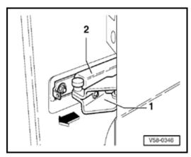
With help from a second technician, guide sliding door back until hinge armature -1-slides out of guide rail -2-.
