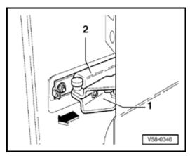
With second technician, guide sliding door back -arrow- until hinge link -1- is out of guide rail -2-.
