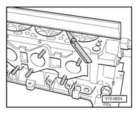
Fig. 1 Cyl. head, checking for distortion
