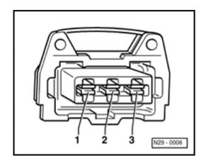
Check for open circuit between Test Box and 3-pin harness connector using wiring diagram, connecting as follows:
