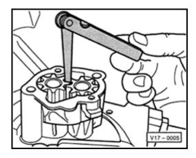
Fig. 1 Oil pump backlash, checking
