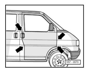
Door is correctly adjusted if, when closed, has uniform gap all around opening, is not sunken, does not protrude, matches contour -arrow-.
