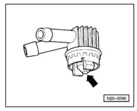
Fig. 2 Gravity/vent valve, checking
