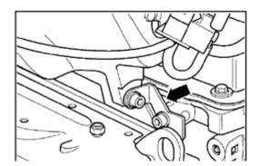
Remove right rear support between intake manifold and cyl. head arrow-.
