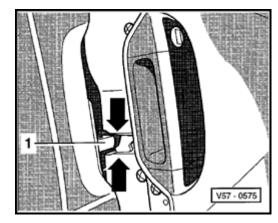
Adjust striker -1- so recess on door lock turn clip is concentric -arrows- to striker (door must not be raised or pressed down). Door must not move when closed.
