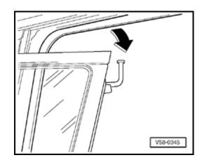
Lower sliding door far enough at front, so that the upper roller guide can be removed from the guide channel.
